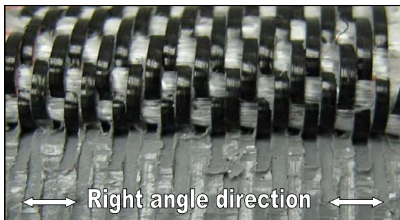
Figure 15: Sample of W-8 with improved peel adhesion on the monofilament polypropylene side, or “black” side.
